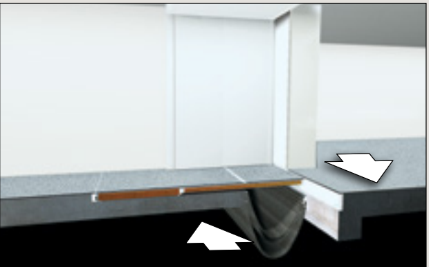
Lateral Shear The cab is attached to the fixed structure by means of a friction-free sliding track assembly to allow full lateral shear between buildings.
