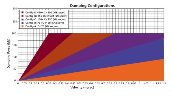
The FVD-B Series dampers are typically utilized on bridge and base isolation platforms requiring a long cycle life. This custom orifice designed damper provides the desired force versus velocity relationship symetrically in both tension and compression directions, thermal compensation, and easy preventative maintenance inspection.
