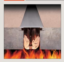
"Sandwich" assembly of layers of stainless steel foil and insulation contained in a stainless steel mesh. Multiflex should be used where lateral shear is required in floor applications having a 3"-12" joint width.
