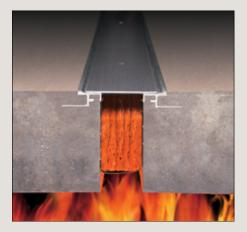
Stainless steel foil drape with block insulation affords maximum economy in material and installation. Wall barriers limited to 1"-4" joints and require no stainless steel foil drape.
